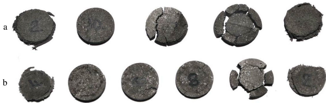
Fig. 7. The appearance of spheroplastic specimens in the initial (a) and aged (b) states after loading without a confining jacket
