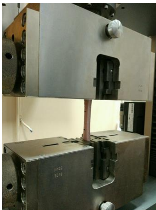
Fig. 5. Material sample in the clips of the testing machine
