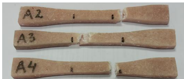
Fig. 6. Destroyed samples after testing
