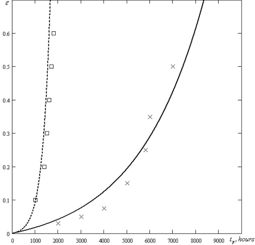
Figure 1: Theoretical creep curves (continuous line - without the account of radiation, dot line - after radiation treatment dose  $1,1 \cdot 10^{21} n/sm^2$ ) of alloy 03X20H45M4BRC at temperature  $650^{\circ}C$ ,  $\sigma = 180 [MPa]$ . Points are data from [9].
