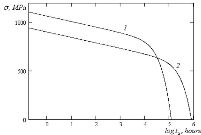
Figure 2: Creep strength curves with the account of radiation (curve 1) and without radiation (curve 2).
