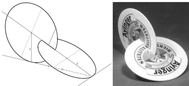
Figure 1: The Two-Circle-Roller and the Oloid.
