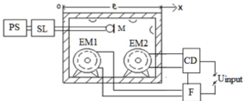
Figure 1: The block diagram of the installation with BSV: EM1, EM2 - electric motors; CD - the circuit of the electric delay; F - the phase-shift network; SL - the sound level meter; PC - the personal computer; M - the microphone
