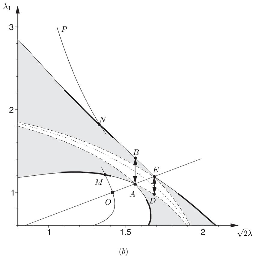
Figure 4: The model material. The PTZ at  $\lambda_2 = \lambda_3 \equiv \lambda$ ;  $ST$  – the line of the uniaxial stretching. (a)  $a = 4.09$ ,  $c_1 = 3$ ,  $c_2 = 1$ ,  $I_c = 4$ ; (b)  $a = 4.4$ ,  $c_1 = 3$ ,  $c_2 = 1$ ,  $I_c = 4$ . The lines  $OM$  and  $NP$  correspond to the path of uniaxial stretching, and the points  $A, B, D, E$  refer to spherically symmetric deformations.
